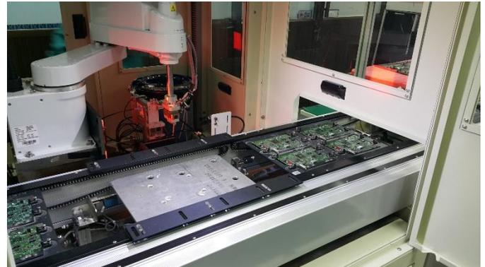
Fig. 5. Machinery industry and Software of robot auto insert project. When feeding printed circuit board in machine.
